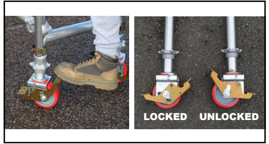
4. Lock Brakes and allow 75mm thread from bottom of castor for levelling
